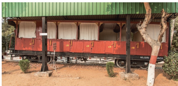
Fig. 17. Third-class coach of the open type (without windows) with separate compartments and individual exterior doors built in the early twentieth century by the Nilgiri Mountain Railway 15 [8]
