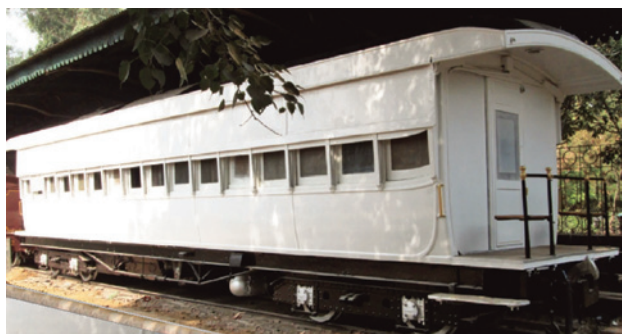
Fig. 15. The wooden Vice Regal Dining Car, painted with white enamel, was built in the Ajmer workshops of BB & CIR (Bombay, Baroda & Central India Railway) in 1889. The carriage was used by the Viceroy of India during his travels around the country and was part of a five-car Vice Regal train. The National Railway Museum, New Delhi [4]
