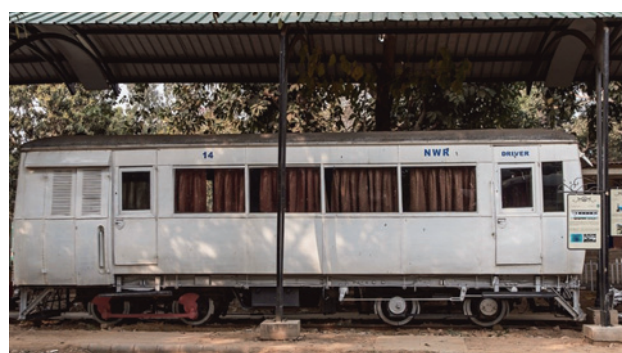
Fig. 20. Railcar RMC 14 of the (762 mm) narrow gauge Kalka-Shimla Railway 17 built in 1933 at Armstrong Whitworth, UR [167]
