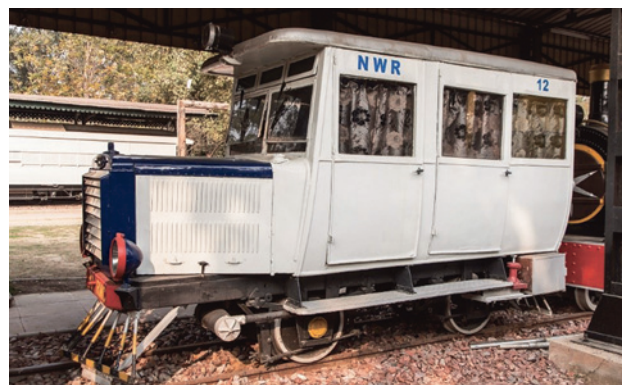
Fig. 19. A twelve-seat railcar of the (762 mm) narrow gauge Kalka-Shimla 17 railway, built in 1931 by Wickham, UR [16]
