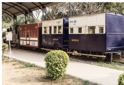
Fig. 16. Coaches (left to right) of the third, first and third classes of the narrow gauge Matheran Light Railway or the Matheran Hill Railway (MHR) with the 620 mm gauge track, 21 km long in the Western Ghats 14 . The line was opened in 1907 and thereafter its operation was suspended several times due to damage caused by natural disasters; however, it has been back to regular operation since November 2012. Matheran Light Railway coaches, Delhi Railway Museum, February 2016 [8]
