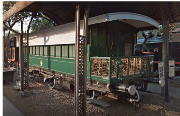
Fig. 8. Broad-gauge coach of Maharaja of Baroda Sayajirao Gaekwad III. Restored by Pratapnagar and Lower Parel Workshop. Complete restoration including electrical equipment, furniture. (Subhabrata) [9]
