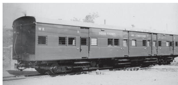
Fig. 25. The metre gauge first/second-class coach of a mixed train of Western Railway (WR). On the photo, the third compartment from the left end of the coach (the third door on the left) is equipped with air conditioning (you can see the inscription 'AIR - CONDITONE' on the wall of the carriage). The ice was loaded into the undercarriage boxes under this compartment. The construction of the carriage is attributed to the mid-1940s. Photo, approx. 1951 27
