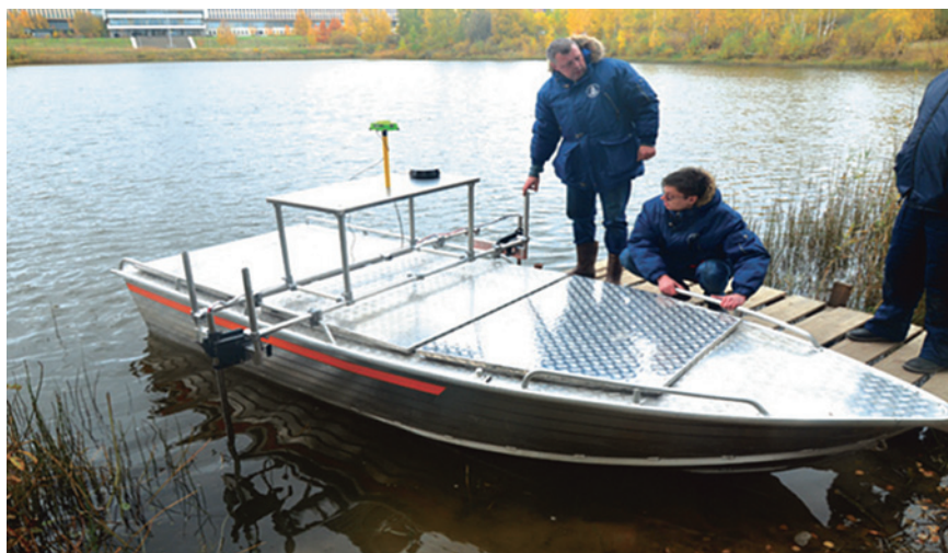
Fig. 5. Experimental vessel with a solar power source
