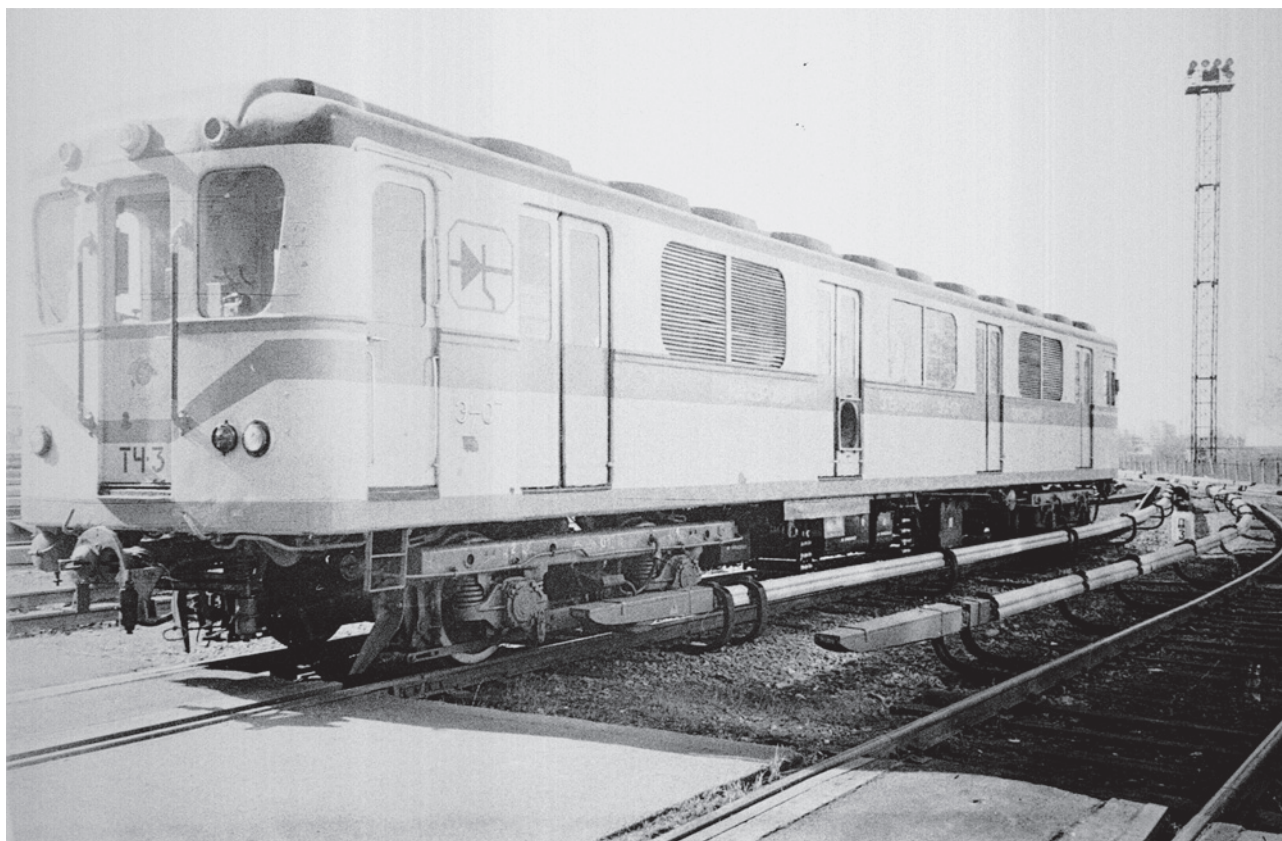
Fig. 3. Battery-trolley electric locomotive for the metro created by the Leningrad Institute of Railway Engineers (currently known as PGUPS) in cooperation with the Ural Electromechanical Institute for Transport (currently known as UrGUPS) and the Design Office of the Leningrad Metro
