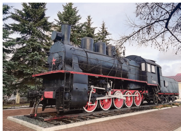
Fig. 3. EU 708-64 (class E, reinforced) 0-5-0 locomotive, factory No. 3482; built at the Bryansk Locomotive Works in 1931.
