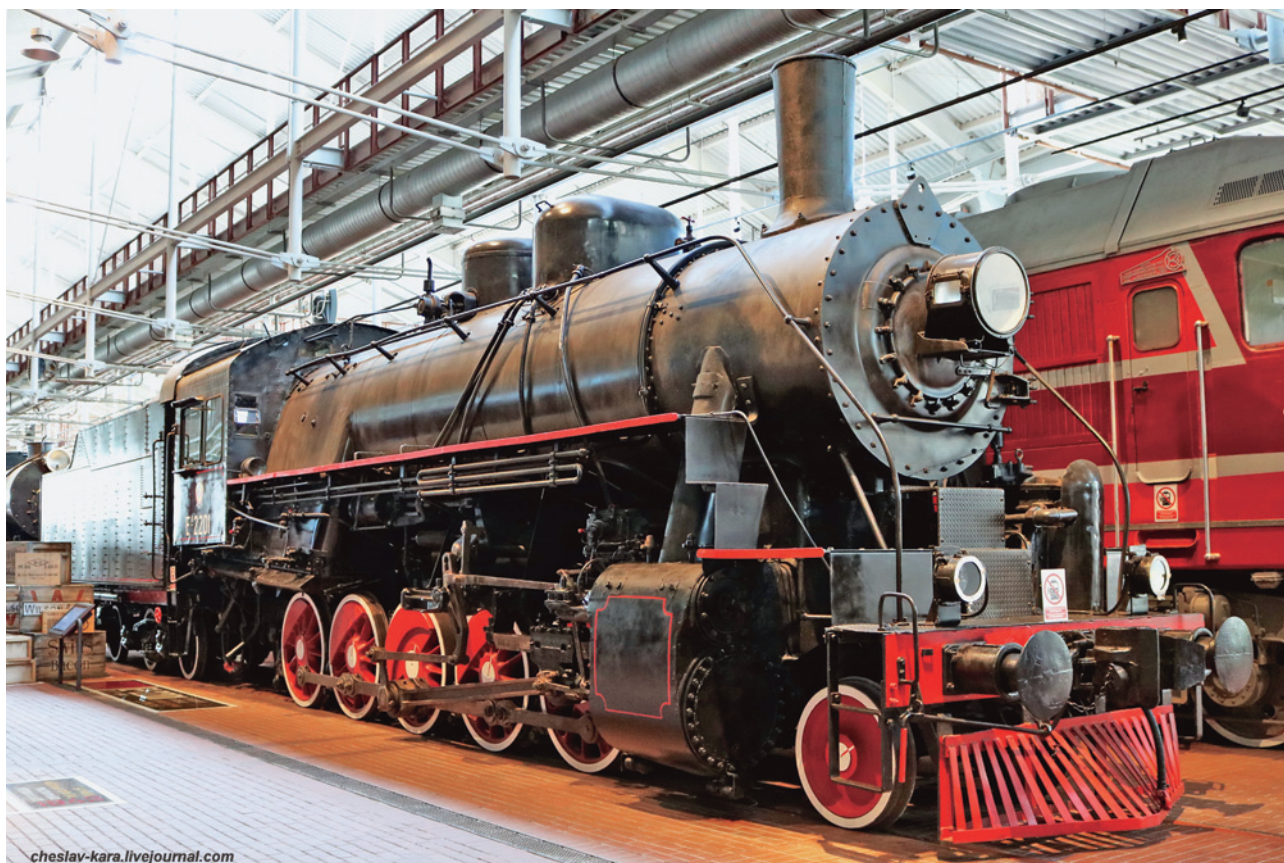
Fig. 1. YeA class 1-5-0 locomotive No. 2201. Built for the USSR under Lend-Lease by Baldwin Works in 1944. From 1944, it was operated on the experimental ring of the Central Research Institute of the People's Commissariat of Railways near Moscow, and in 1955 it began to be used on the Far Eastern Railway. In 1992, the locomotive was moved from the Vyazemskaya depot of the Far Eastern Railway to the October Railway Museum in St. Petersburg (currently the Museum of Russian Railways) 9
