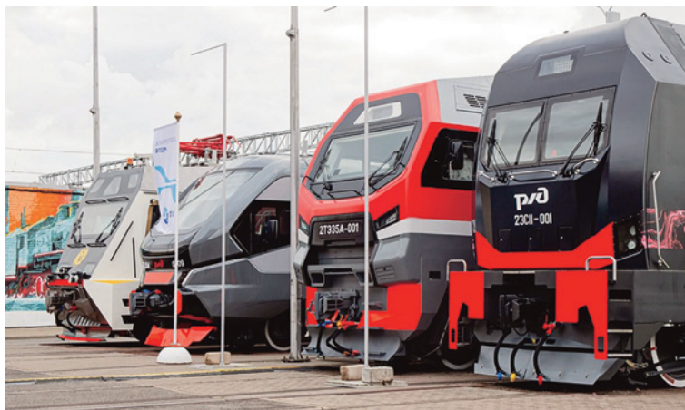
The newest Russian locomotives and wagons: In the photo from left to right: a two-section multifunctional diesel vehicle of the Pioneer-Integral project, designed to diagnose infrastructure devices, by JSC Firma Tvema; EP2M suburban DC electric train by Demikhovo Machine-Building Plant; two-section electric locomotive with asynchronous traction electric motors 2TE35A by JSC Sinara – Transport Machines; main cargo electric locomotive of alternating current 2ES11 "Orlets" with asynchronous traction drive by Ural Locomotives LLC. Photo Photobank of JSC Gudok Publishing House
