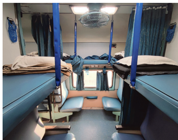
Fig. 9. Interior of a bay on a 2AC coach. View from the four transverse sleeping berths to the two longitudinal berths, with the lower berths converted to seats during the daytime. Photos courtesy of Nonstop Eurotrip [8]
