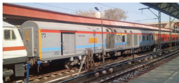
Fig. 3. LHB carriage with an electric generator and luggage compartment. Photo by the authors. March 2019
