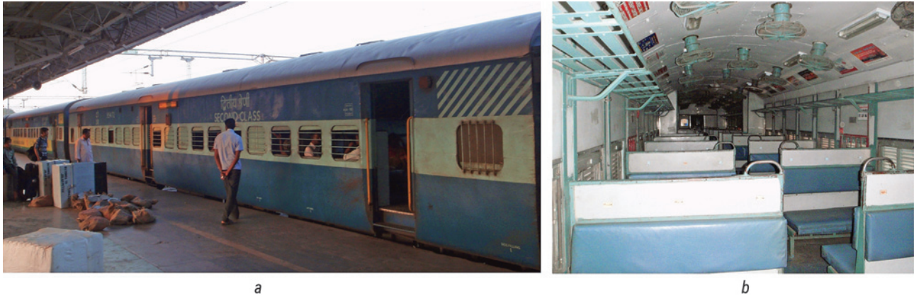
Fig. 13. Non-air-conditioned second class (2S) ICF coach: a – exterior of a train at the platform before boarding (the luggage ready for loading); b – interior of a coach with benches, each for three passengers. Photo by the authors, 2013
