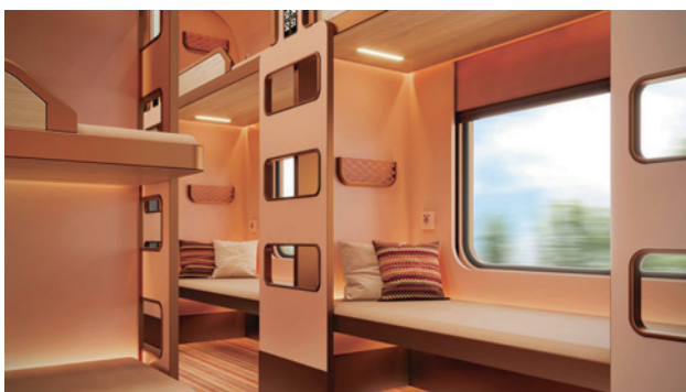
Fig. 7. Interior of a Vande Bharat sleeper coach designed by Kinet Railway Solutions. The coach has an open-plan layout with two-tiers of berths for passengers (similar to a Russian-style "reserved seat" coach). Design presentation 13
