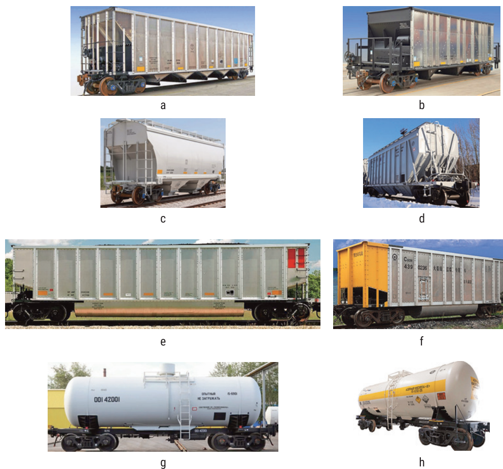
Fig. Aluminium alloy cars from different countries: a – Aluminum AutoFlood III (USA); b – Steel and Aluminum Triple Hopper Aggregate (USA); c – Small Cube Covered Hopper (USA); d – hopper car, model 19-1299 (Russian Federation); e – Aluminum BethGon II (USA); f – 1060 mm gauge C80H Aluminum Alloy Coal Gondola (PRC); g – tank car, model 15-6901 (Russian Federation); h – tank car, model 15-1232-05 (Russian Federation)
