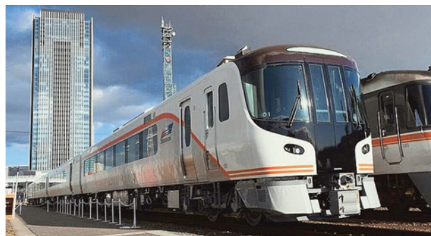
Fig. 12. Train with hybrid propulsion system of HC85 series
