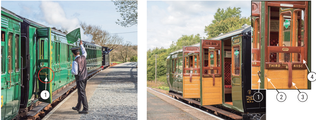
Fig. 14. Preserved third-class standard gauge carriages with compartments occupying the width of the carriage body on the historic Isle of Wight Steam Railway, UK. The individual outside doors of each compartment open outwards. The photo clearly shows that the side of the door facing the inside of the carriage (the right photo, an enlarged detail of the door) does not have a handle to open the door lock (2), it is only available on the outside (1), which is clearly visible in the left photo. On the right photo: 3 – a traditional for British carriages strap for lifting the movable glass of the door window; 4 – the movable glass of the carriage door window [18]. To open the door the passenger had to stick his hand out of the window and turn the handle of the door lock from the outside to open it
