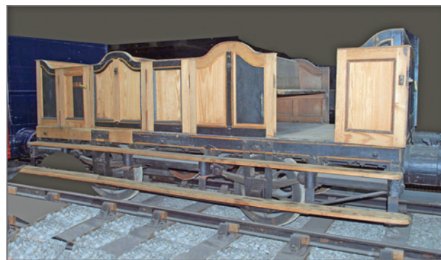
Fig. 4. Bodmin & Wadebridge Railway third-class open carriage. Cornwall's first steam railway, 1834. One of the three earliest surviving coaches of England's first railways. The National Railway Museum, York. Photo: Hugh Llewelyn. [8]. Figure 6 shows coaches of this type of the Liverpool and Manchester Railway
