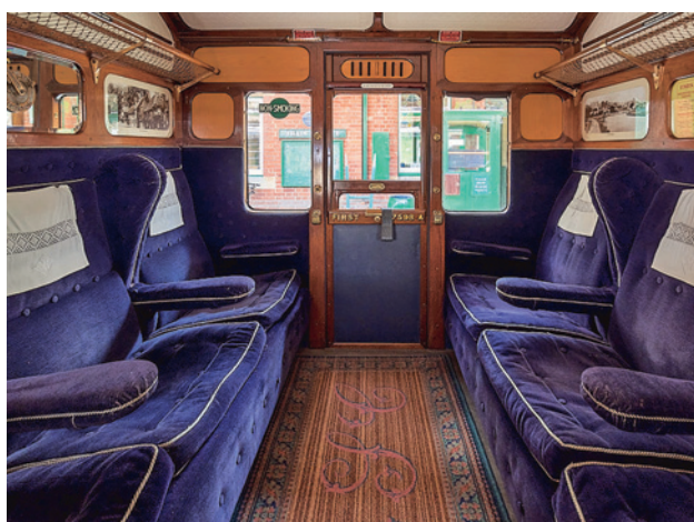
Fig. 12. First-class compartment (separated from other compartments in the coach) with its own external doors. The historic Bluebell Railway. The Bluebell Railway is a heritage line. UK. The authors have already noted the lack of handles on the inside of the doors to open the door lock. In order to open the door, a passenger had to turn the handle on the outside of the door by sticking his hand through the open window 9
