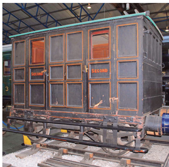
Fig. 3. Enclosed coach with two separate compartments with doors opening outwards. Bodmin & Wadebridge Railway – Cornwall's first steam railway. 1834. One of the three surviving coaches from England's first railways. The National Railway Museum, York. Photo: Hugh Llewelyn [8]
