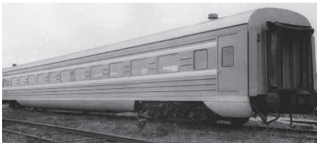
Fig. 9. The RT200 carriage "Russian Troika". Troika (rus. – Troika) – a vehicle (sleigh or wheeled carriage) drawn by three horses. 1974 [11]
