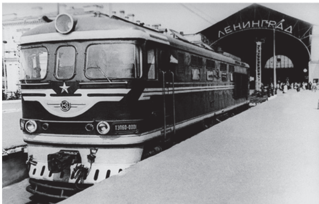
Fig. 6. The first high-speed diesel locomotive TEP60-001, 1961 [11]
