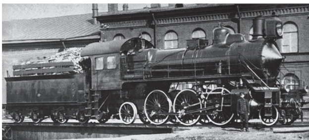
Fig. 2. Steam locomotive type 1-3-1 of S series of the first series at Nikolaevskaya Railway, 1915 [11]
