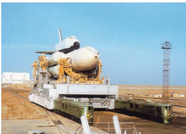
Fig. 4. Assembled full-scale mock-up of RN (rus. PH) Energy booster: 4M item in the process of transportation with ПТЭ3 diesel locomotives
