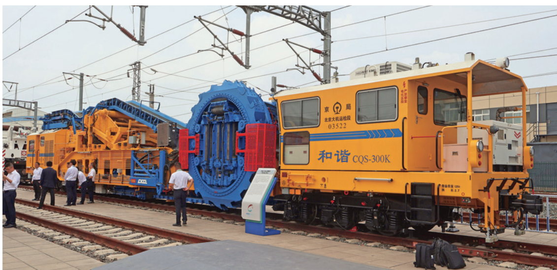
Fig. 20. China's new CQS-300 ballast cleaning machine intended for operations on turnouts with 4,800 mm reinforced concrete turnout sleepers. Photo by the author
