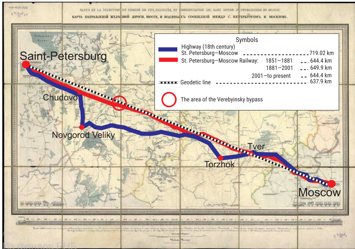
Fig. 3. Map of directions of railways, highways and water ways between St. Petersburg and Moscow The map shows the line of the St. Petersburg–Moscow railway under construction. With supplements by Igor P. Kiselev 4 [6]
