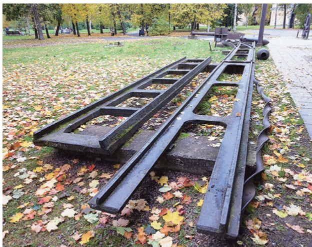
Fig. 2. Surviving iron-cast wheel tracks of the trackway at the Aleksandrovsky Factory in Petrozavodsk. Permanent exhibition of the National Museum of the Republic of Karelia. 2017. Photo by Mikhail Semenov 1
