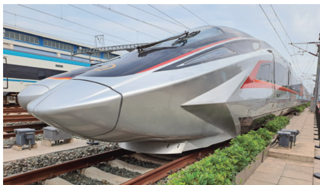
Fig. 22. China's experimental CR450 AF high-speed electric multiple unit with the design speed of 450 km/h. You can clearly see the stamped three-dimensional silhouette of an arrow on the hull plating – an element of the train brand. Photo by the author
