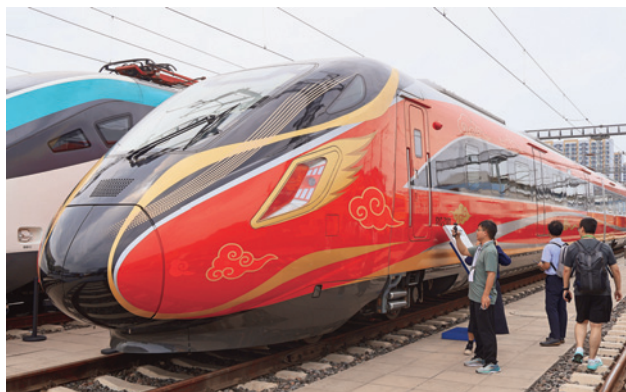
Fig. 21. China's eight-carriage high-speed electric multiple unit for suburban and urban services with the design speed of 200 km/h. It can accommodate 1,592 passengers in seating. Photo by the author
