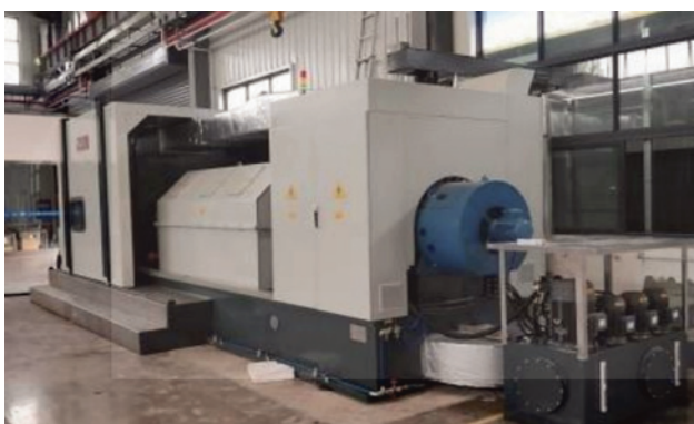
Fig. 19: a – General view of the testing facility for braking equipment; b – Test unit for brake discs and brake assembly
