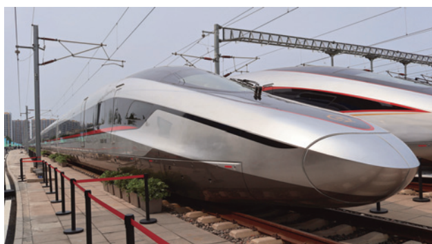
Fig. 23. China's experimental CR450 BF high-speed multiple unit with the design speed of 450 km/h. The designers' idea is that the nose fairing of the driving trailer should look like a falcon beak – an element of the train logo. Photo by the author
