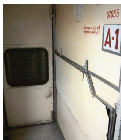
Fig. 17. Non-air-conditioned 2S ICF coach. Entrance vestibule. Folding berth for an on-duty attendant. Photo by the authors. 2019
