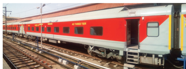
Fig. 2. LHB coach with air conditioning and three-tier sleeping berths (3AC) (with reserved seats). Photo by the authors. March 2019
