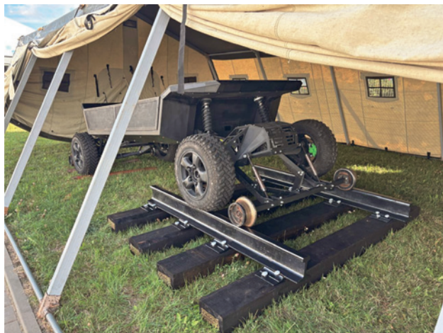
The unmanned platform on a combined course "Sputnik-ZhD" (Sputnik railway platform) that was developed by specialists from Emperor Alexander I Petersburg State Transport University's Department of "Ground transport and Technological Complexes". Photo by Tatiana Arzamastseva
