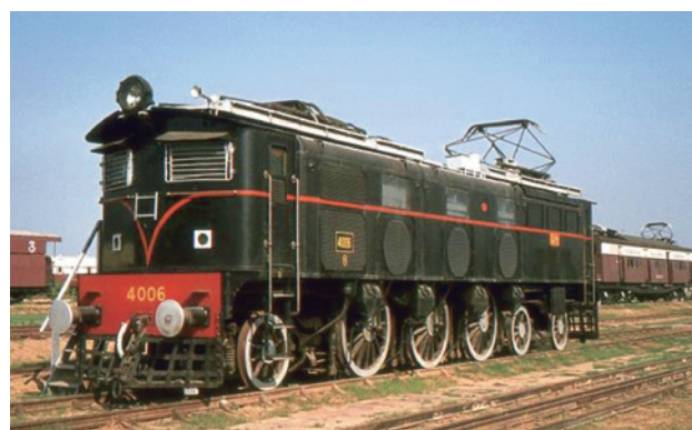
Fig. 8. The Sir Roger Lumley electric locomotive, commissioned in 1930, was the first passenger electric locomotive of the Indian Railways. A 1.5 kV DC, type 1-2-2 machine, originally given the serial name EA/2, later renamed WCP-2, preserved in the National Railway Museum, New Delhi. It is believed that this particular electric locomotive was part of the first Deccan Queen train to enter the route on June 1, 1930 14
