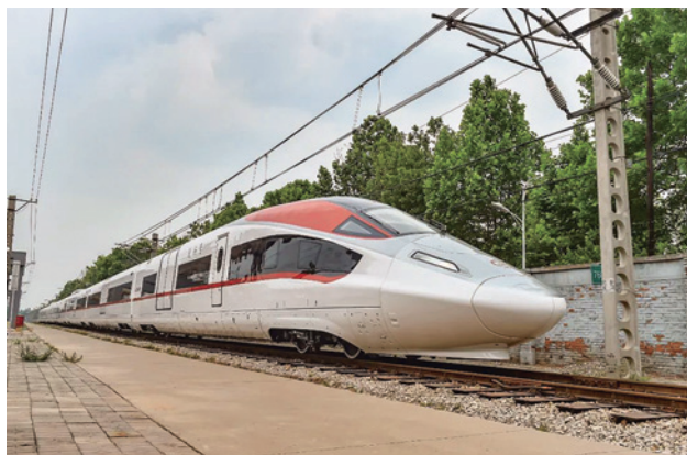
Fig. 2. The world's first Chinese high-speed freight train with a design speed of 380 km/h, based on the latest generation of Fuxing high-speed passenger trains, is seen during a presentation at the Tangshan factory of CRRC Tangshan Co, Ltd. in Tangshan, Hebei province, on December 23, 2020 (Railway Transport. 2021. No. 11. P. 69)
