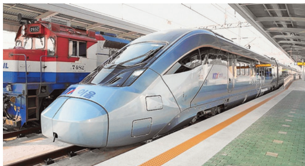
Fig. 11. High-speed electric train with distributed traction KTX-Eum
