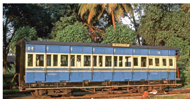
Fig. 13. First/second class mixed metre-gauge coach of the Indian Railways with separate compartments, without a passage (corridor) along the coach body, with each compartment having its own external door. First class compartments – the two outermost doors on the right are labelled “A” and “B” (the letters are shown below the Roman numerals indicating the compartment class). The Nilgiri Mountain Railway is recognised by UNESCO as a world cultural heritage site. The coach has a route plate with the name of the city to which the train is travelling: Mettupalaiyam (in the Coimbatore district of the Indian state of Tamil Nadu). The coach was built in the 1960s. The historic railway is operated for excursion and tourist activities 10
