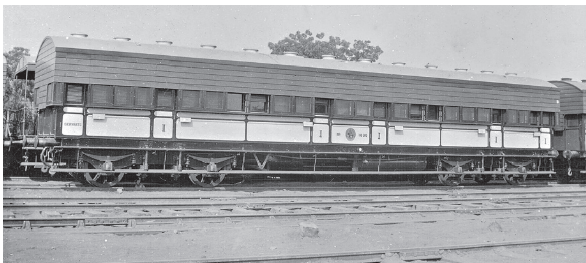
Fig. 15. India Railways – Great Indian Peninsula Railway - GIPR First Class passenger coach with separate compartments and individual entrance doors (no corridor). The door on the far right is probably for a single compartment; the door on the far left labelled “Servants” leads to a service room; the door on the right is probably to the largest compartment designed for several passengers. On the photo you can see that the upper part of the carriage is covered with wooden boards, the so-called “planking”. There was a gap between the planking and the wall which was blown with air to reduce heating of the upper part of the coach by sun rays. The end of the 19th century 13
