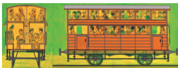
Fig. 10. Bombay, Baroda and Central India Railway's third-class double-axle double-decker open carriage. (Image: Getty Images) 1860s. A section of the carriage clearly shows that the first floor, where the stairs led to, has a low ceiling, which allowed passengers to bend down to pass or sit on the benches [12]
