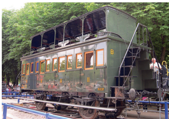
Fig. 9. A preserved historic double-decker double-axle carriage with the imperial of the French railways. The ground floor of the carriage has four eight-seat compartments occupying the full width of the carriage body, each with individual exterior doors. The 36-seat imperial (first floor) is an open compartment (without side walls) with wooden benches 7
