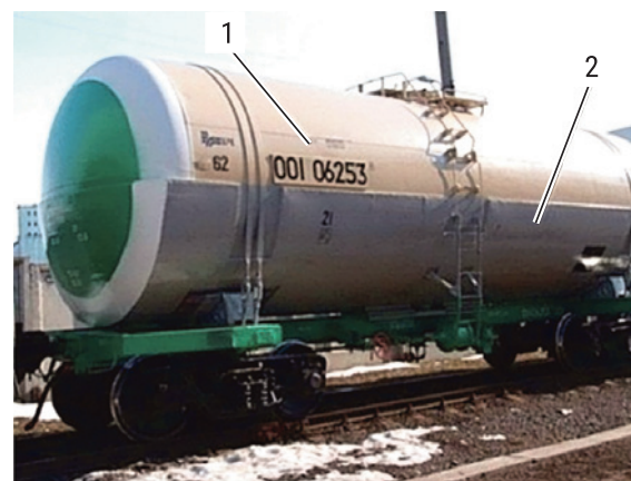
Fig. 5. Tank wagon with a steam heating casing, model 15-1566: 1 – tank of the tank wagon; 2 – steam heating casing of the tank
