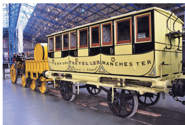
Fig. 2. Passenger rolling stock of the first railways. Liverpool and Manchester Railway coaches – the first class. England. 1830. The National Railway Museum, York, England. The coach has three isolated compartments with individual doors that open outwards. The exterior colouring of the car emphasises the continuity with the design of a stagecoach body: the impression is that three carriages are placed on the carriage frame [7]
