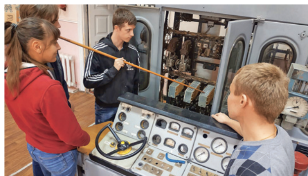
Students at classes in the laboratory of the Railway Rolling Stock Department. Training simulator: High-voltage cabinet and control console of 2TE116 diesel locomotive
